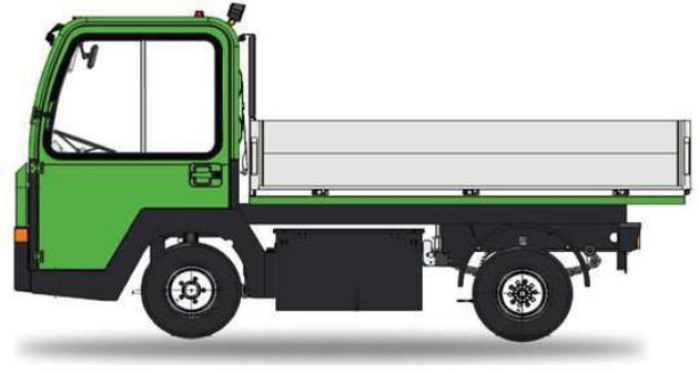
4-wheel platform truck, man on board, with rear-wheel drive. Extremely easy to drive, ideal for all duties - both indoors and outdoors, even on long distances. The platform of the PE30 truck can be completed with other equipment.
