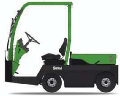
4-wheel tow tractor, man on board, with rear-wheel drive. Extremely easy to drive, ideal for all duties - both indoors and outdoors. Ideal solution whenever the operator has to get off frequently for hooking and unhooking operations. Loading capacity of rear platform 100 kg.
