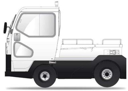
4-wheel tow tractor, man on board, with rear-wheel drive. Ideal for all intense duties - both indoors and outdoors. Loading capacity of wide rear platform 200 kg.
