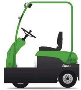
3-wheel tow tractor, man on board, with rear-wheel drive. Extremely compact and easy to drive, ideal for all industrial duties - both indoors and outdoors.
