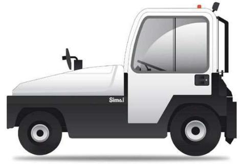
4-wheel tow tractor, man on board. Heavy-duty high-performance and long-range truck for industrial and airport duties. Despite its small size and turning radius, the TE300R has a high towing capacity. Driving position is located backwards ensuring optimum weight distribution and excellent stability. Loading capacity of front platform 80 kg.
