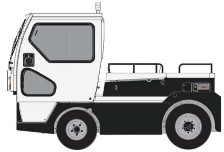
4-wheel tow tractor, with on-board operator. Heavy-duty high-performance and long-range truck for industrial and airport duties. Despite its small size and turning radius, the **TE252** has a 25-tonne towing capacity. **TE293** version with 29-tonne towing capacity. Loading capacity of wide rear platform 200 kg.
